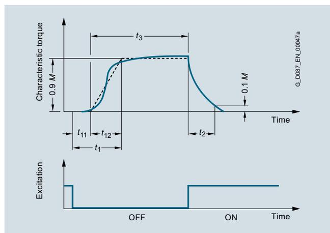
Fig. 2/19 Brake switching times
