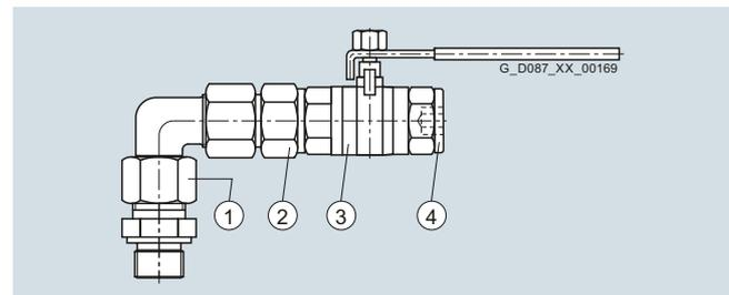
Fig. 10/22 Oil drain valve, angled
