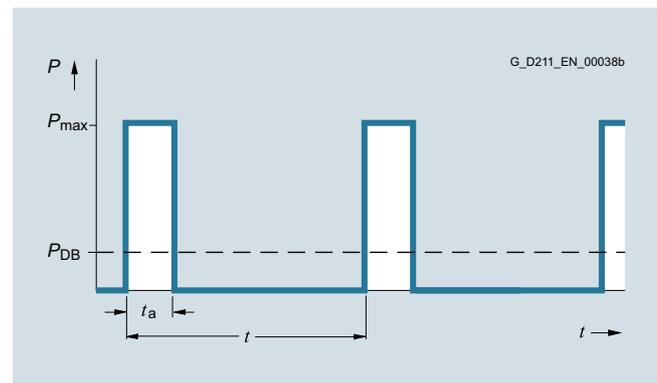
Fig. 9/23 Load diagram for braking resistors
