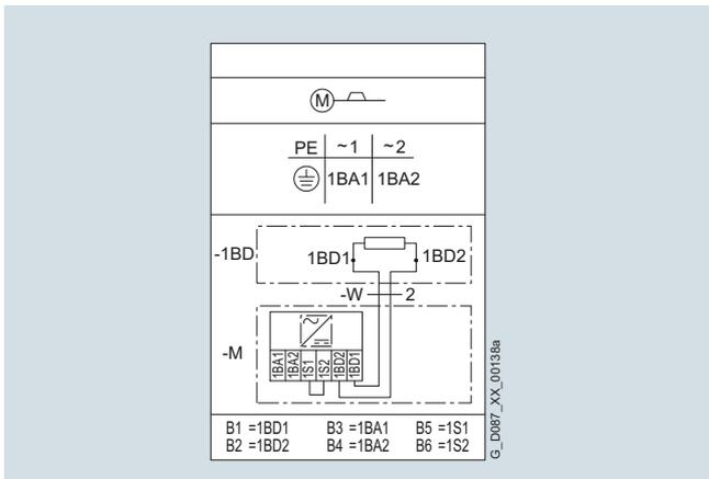
Fig. 11/32 Connection circuit diagram with AC control voltage
