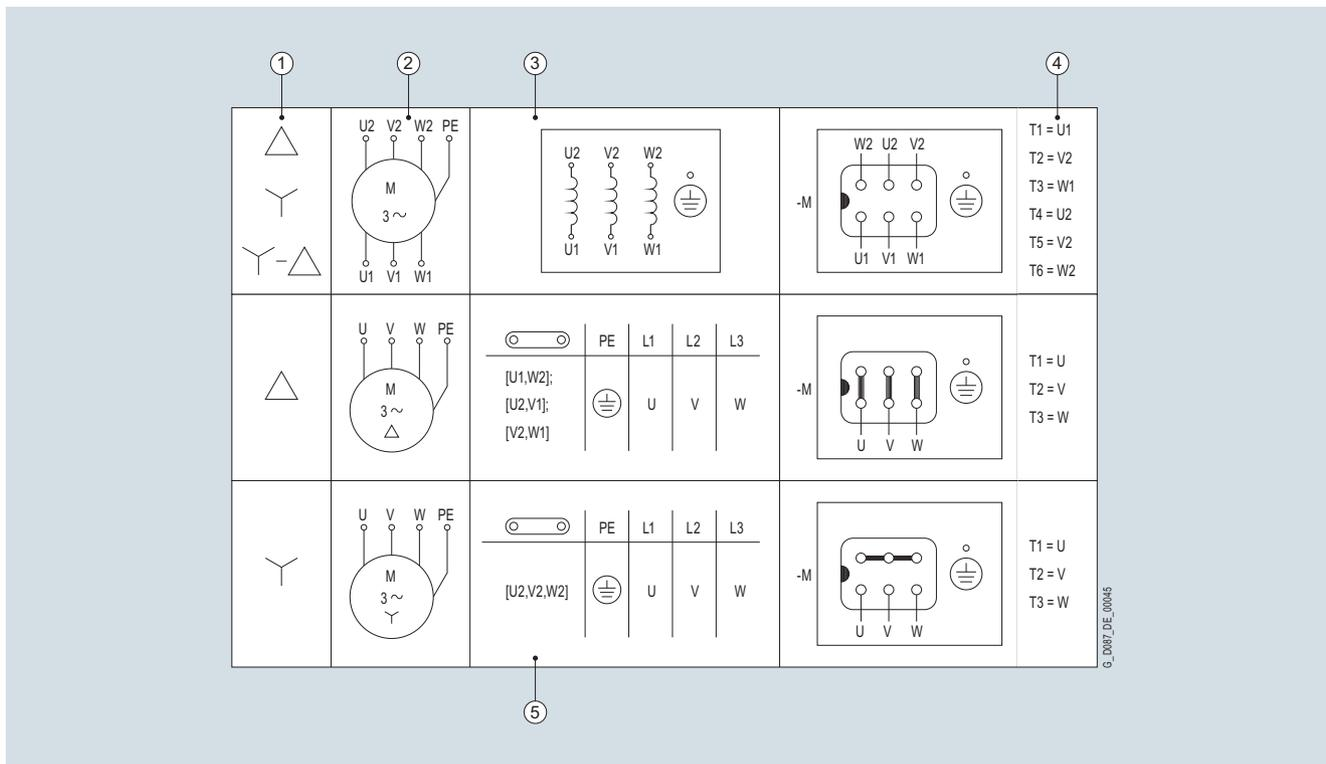
Fig. 11/9 Connection circuit diagram, motor connection  $\Delta/Y$
