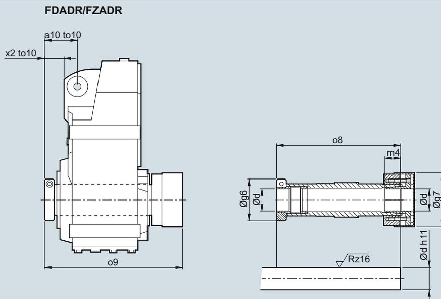
Note mounting tolerance to10 when positioning the torque arm.
