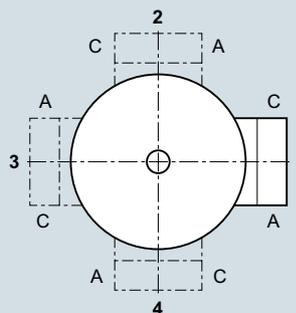
Fig. 11/8 Terminal box position and cable entry
