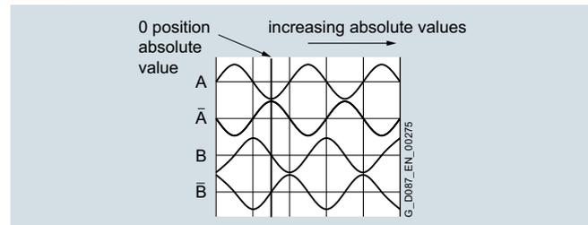
Fig. 11/53 Chart pattern with shaft rotating in clockwise direction (looking in direction of clamping ring)
