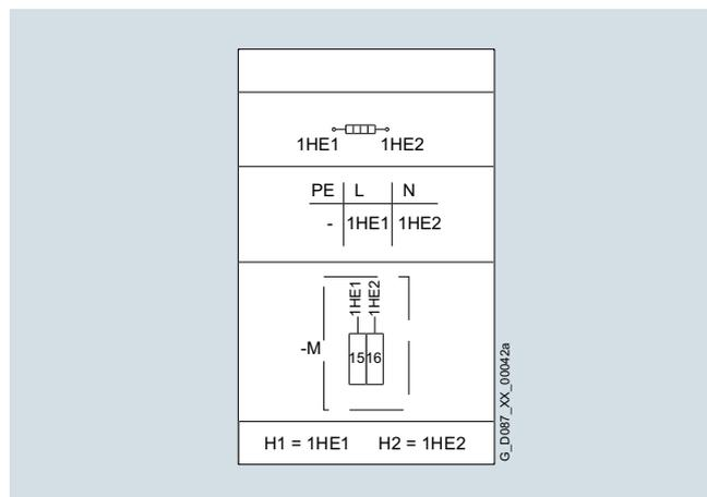
Fig. 11/7 Connection circuit diagram for the anti-condensation heating
