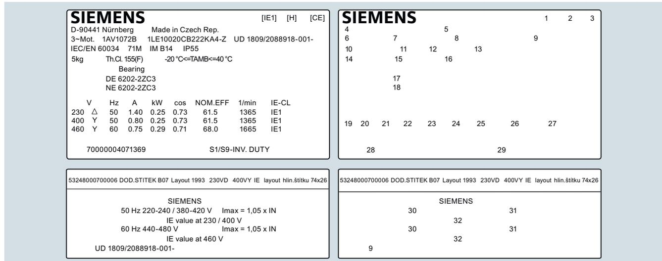
Fig. 12/6 Example of a rating plate on the motor side on worm geared motor S
