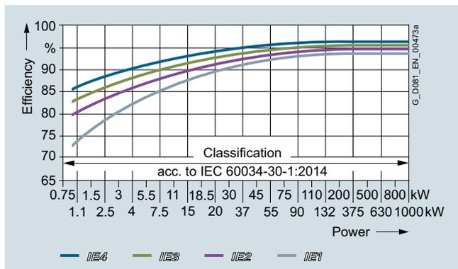
Fig. 1/18 IE1-IE3 efficiencies 4-pole at 50 Hz
