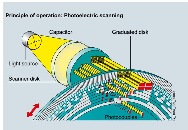
Fig. 2/26 Principle of operation, photoelectric scanning
