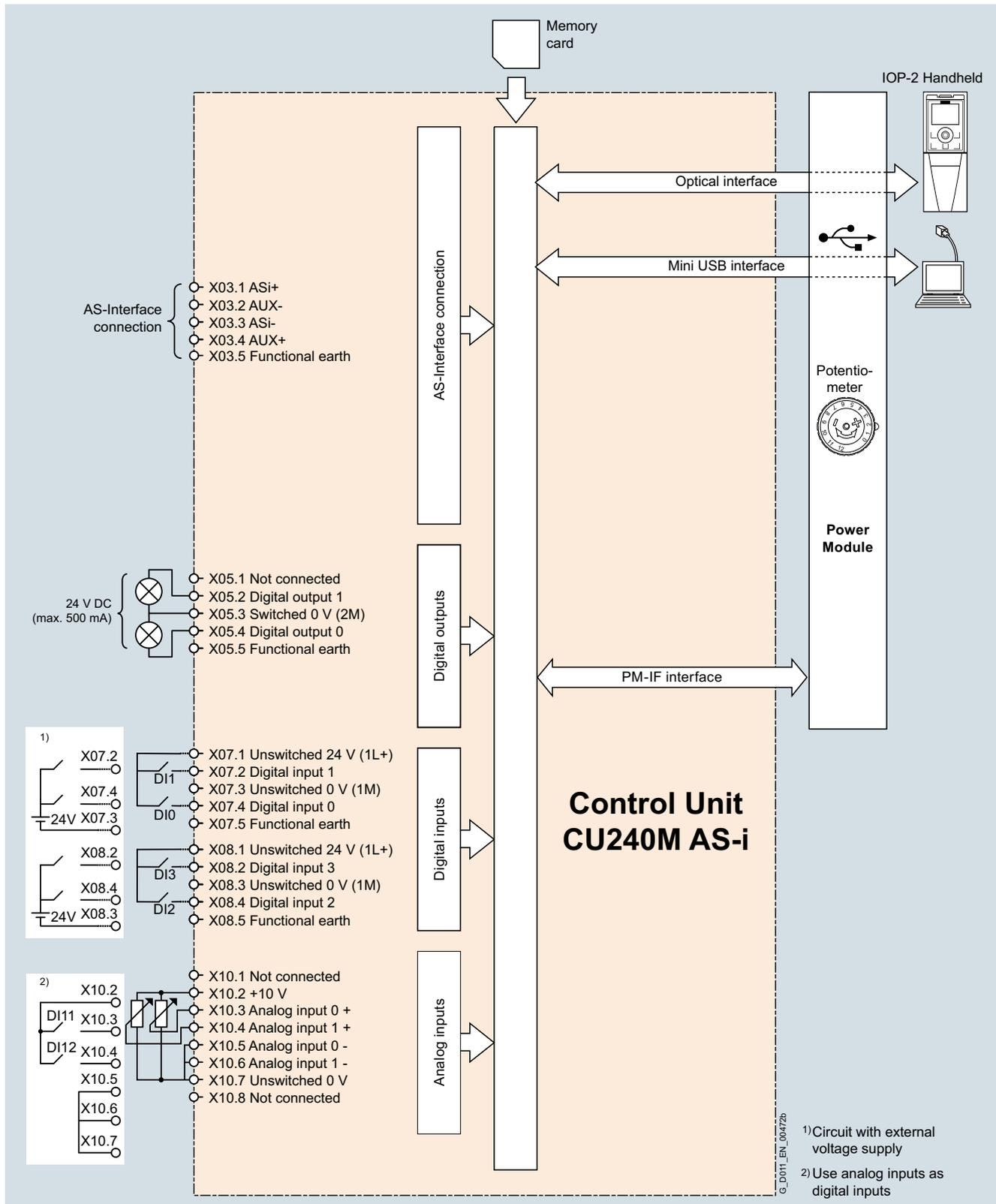
Fig. 9/10 Connection diagram for CU240M AS-i Control Units
