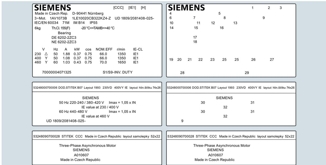
Fig. 12/7 Example of a rating plate on the motor side in CCC design on worm geared motor S
