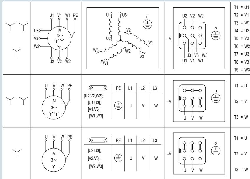
Fig. 11/11 Connection circuit diagram, motor connection YY/Y
