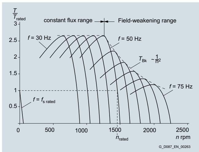
Fig. 2/29 Example for a 4-pole, three-phase asynchronous motor
