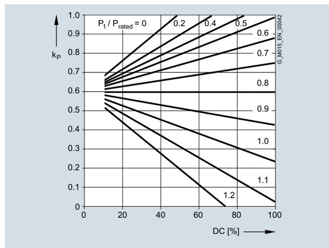
Fig. 2/18 Power requirement and duty cycle
