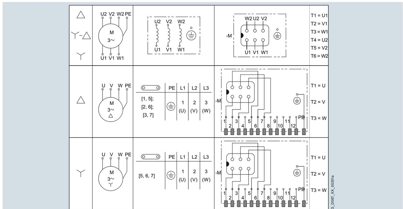
Fig. 11/29 Connection circuit diagram for motor winding
