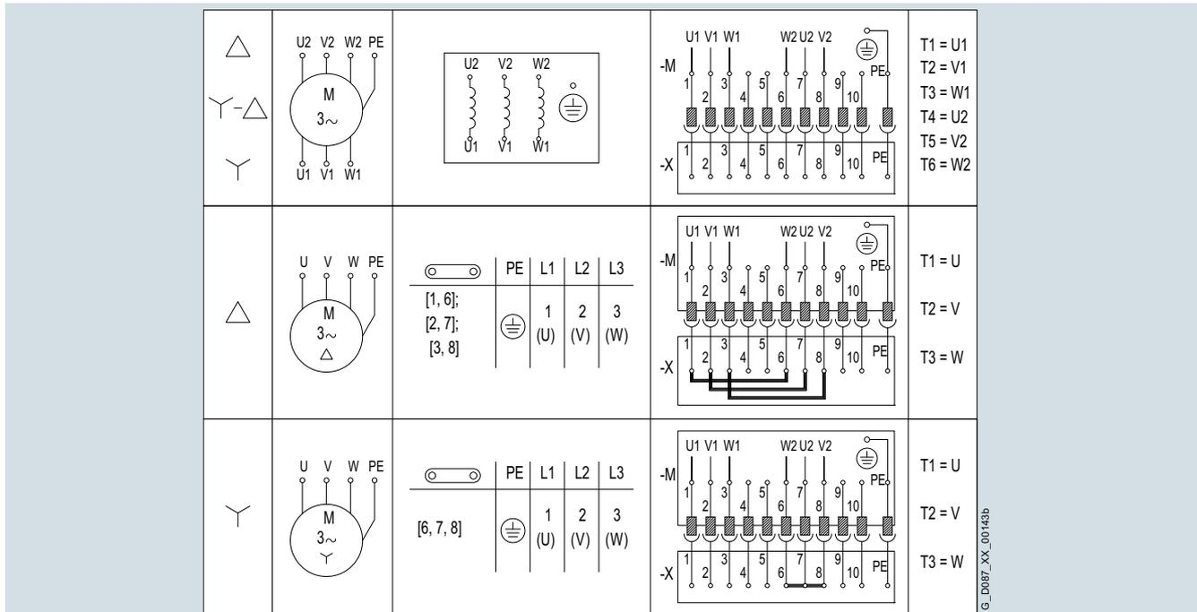
Fig. 11/15 Connection circuit diagram for motor winding
