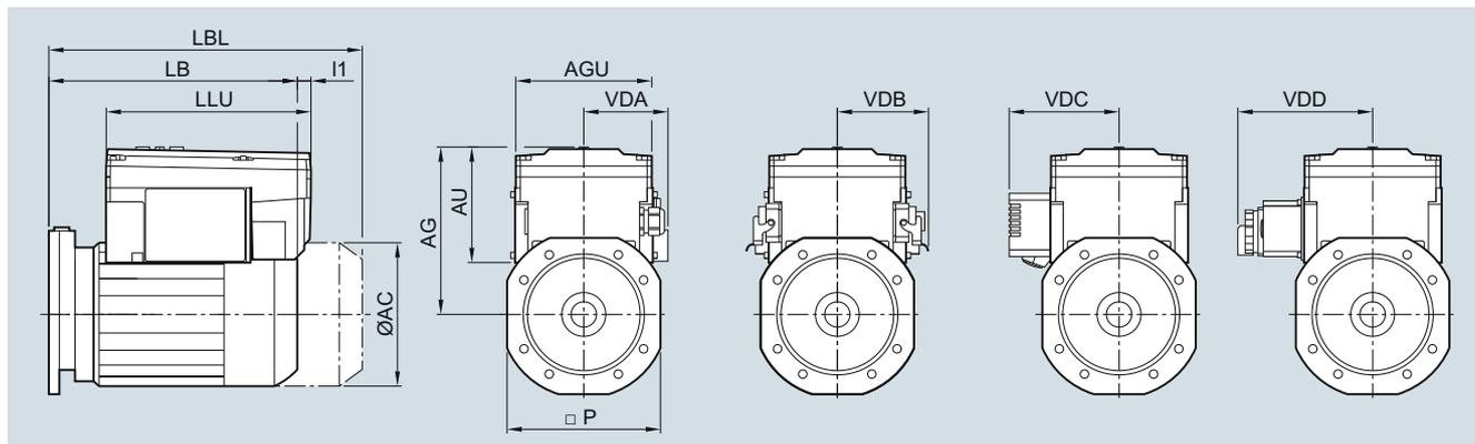
The diagram is for terminal box position 2A (for further information about the terminal box position, see [page 11/16](#)).
