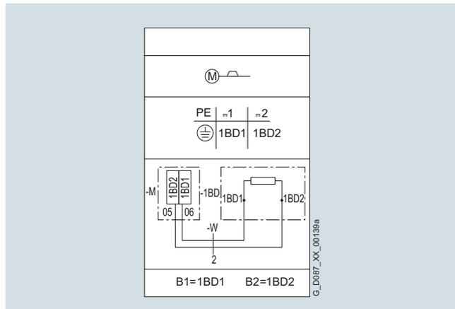
Fig. 11/33 Connection circuit diagram with DC control voltage
