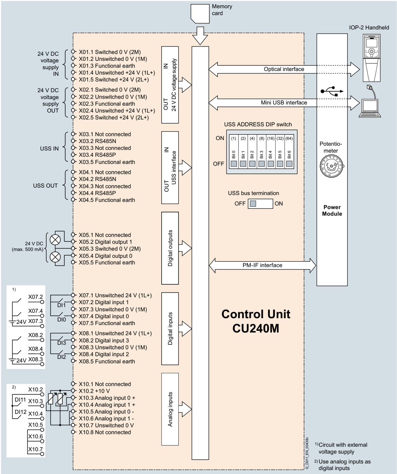
Fig. 9/9 Connection diagram for CU240M Control Units
