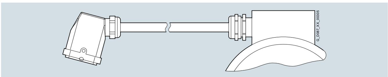
Fig. 11/23 HAN Q8 motor plug with cable
