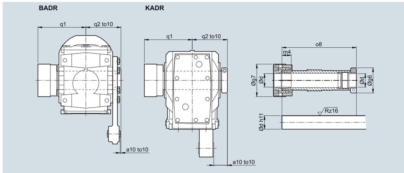
Note mounting tolerance to10 when positioning the torque arm.
