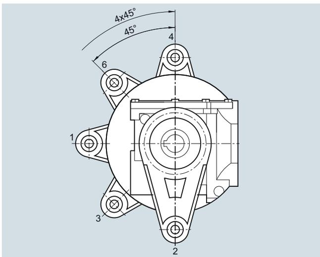
Fig. 10/10 Helical worm gearboxes CAD, size 29
