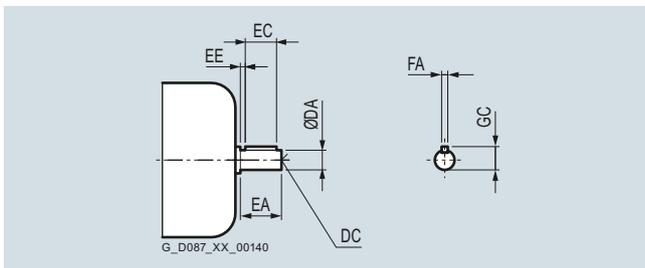
Fig. 11/57 Second motor shaft extension
