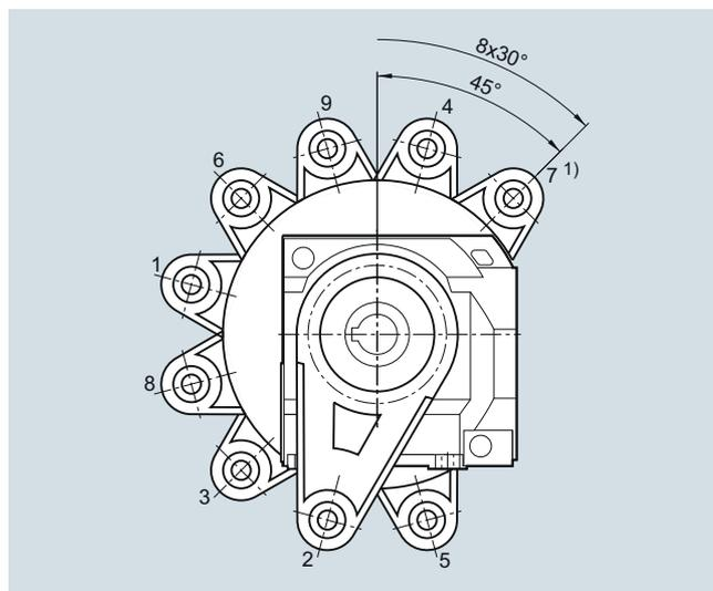
Fig. 10/12 Helical worm gearboxes CAD, Figure 2, sizes 39 to 89
