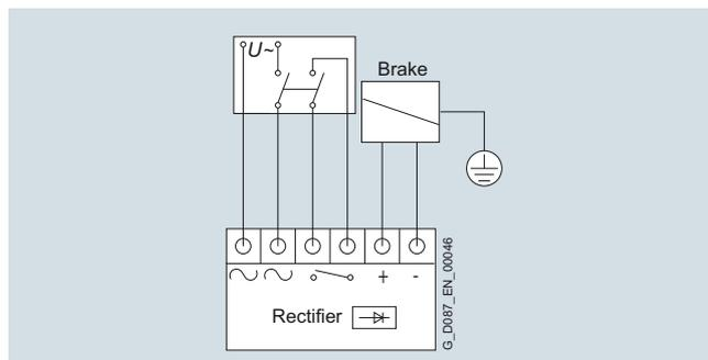
Fig. 11/35 Function diagram of a brake switched on the DC and AC sides
