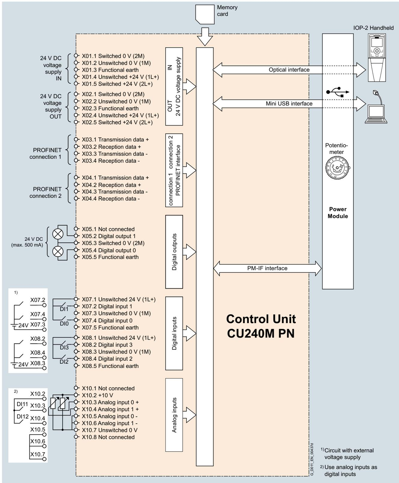
Fig. 9/12 Connection diagram for CU240M PN Control Units
