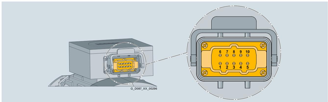
Fig. 11/14 HAN 10E motor plug with pin assignments
