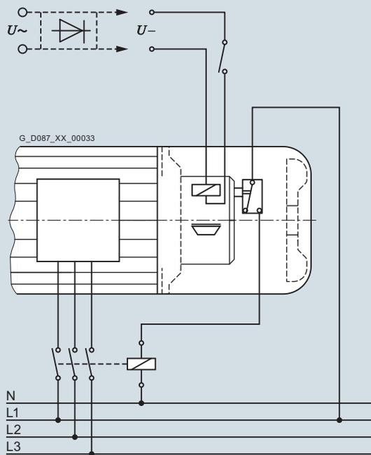
Fig. 11/43 Circuit principle with microswitch
