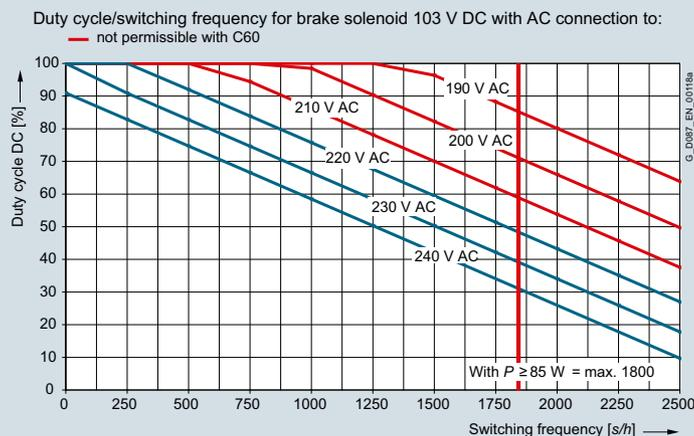
Fig. 11/36 Duty cycle factor/switching frequency for the 103 V DC brake solenoid
