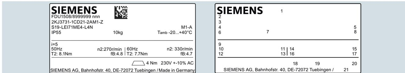
Fig. 12/5 Example of a rating plate on gearbox side on worm geared motor S
