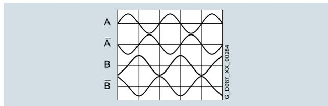
Fig. 11/51 Chart pattern with shaft rotating in clockwise direction (looking in direction of clamping ring)
