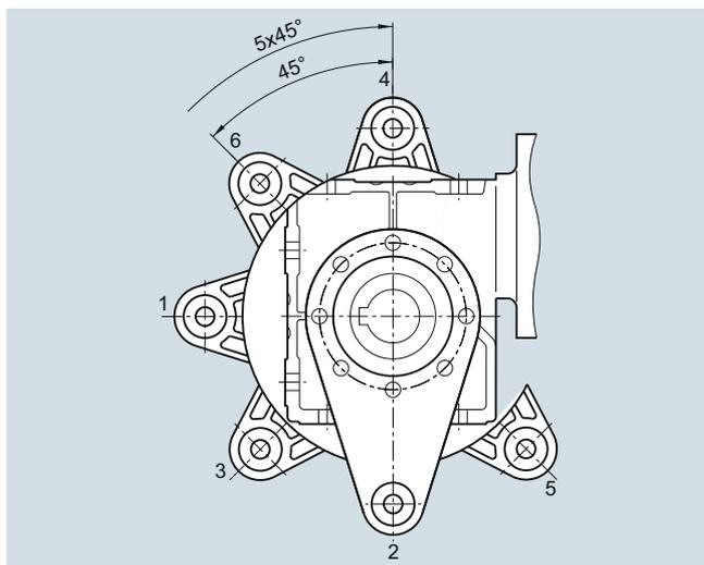
Fig. 10/13 Worm gearboxes S in a shaft-mounted design
