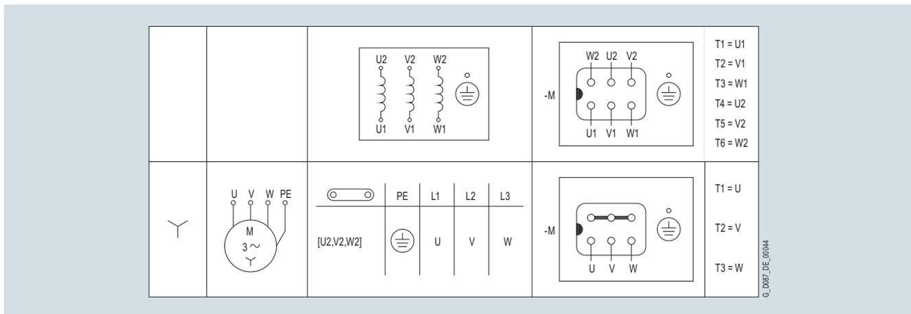
Fig. 11/10 Connection circuit diagram, motor connection Y
