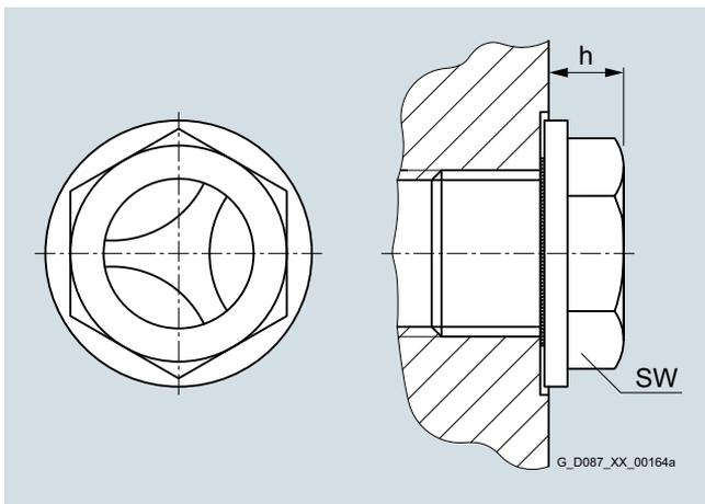
Fig. 10/20 Oil sight glass with reflector
