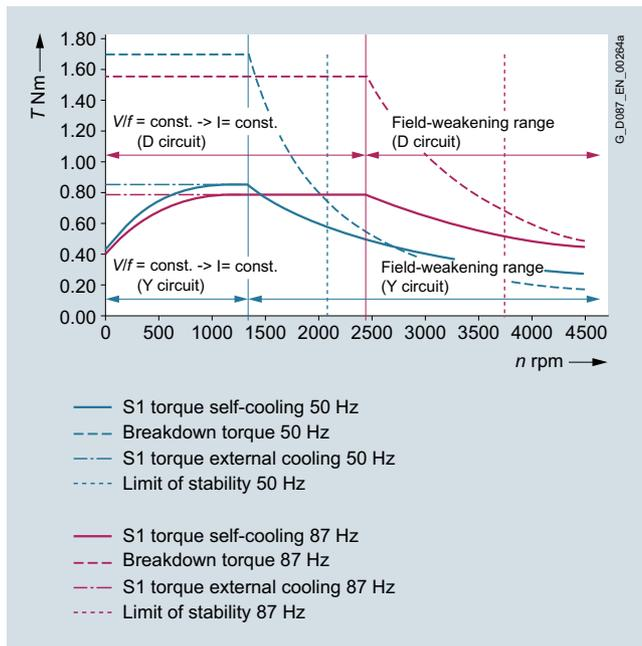
Fig. 2/30 Example of torque-speed characteristic of a 4-pole asynchronous motor
