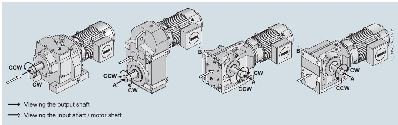
Fig. 1/19 Definition of the direction of rotation
