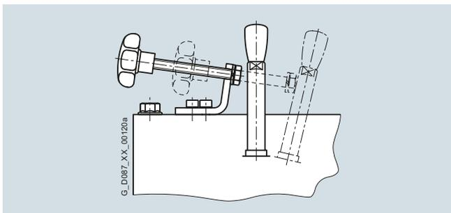
Fig. 11/39 Example of manual brake release lever with locking mechanism for brake L
