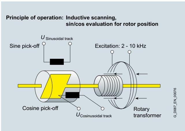
Fig. 2/24 Principle of operation, inductive scanning
