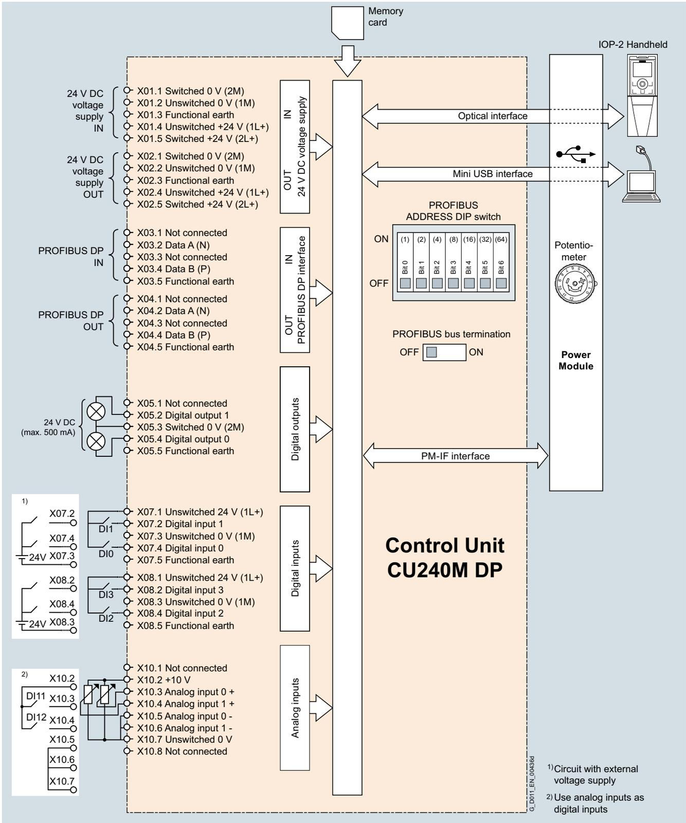
Fig. 9/11 Connection diagram for CU240M DP Control Units
