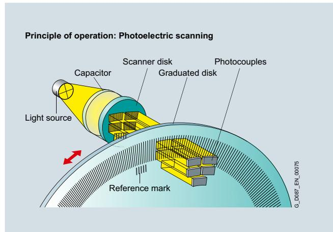
Fig. 2/21 Principle of operation, photoelectric scanning
