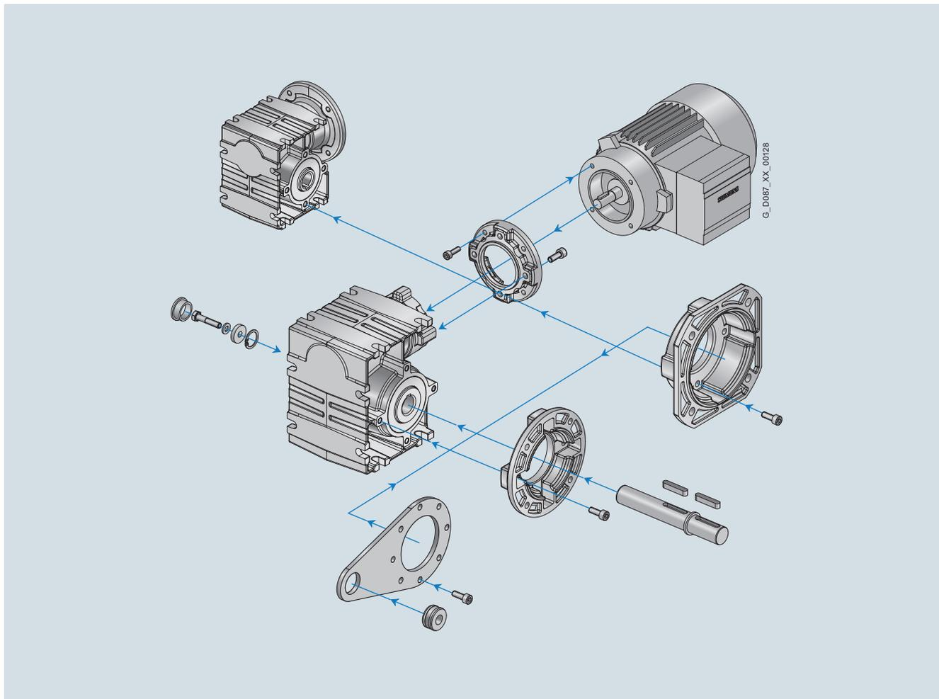
Fig. 1/16 Modular system, worm gearbox
