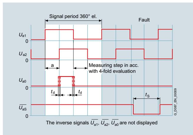
Fig. 2/23 Inverse output signals
