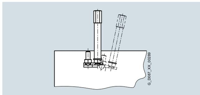
Fig. 11/40 Example of manual brake release lever with locking mechanism for brake FDX
