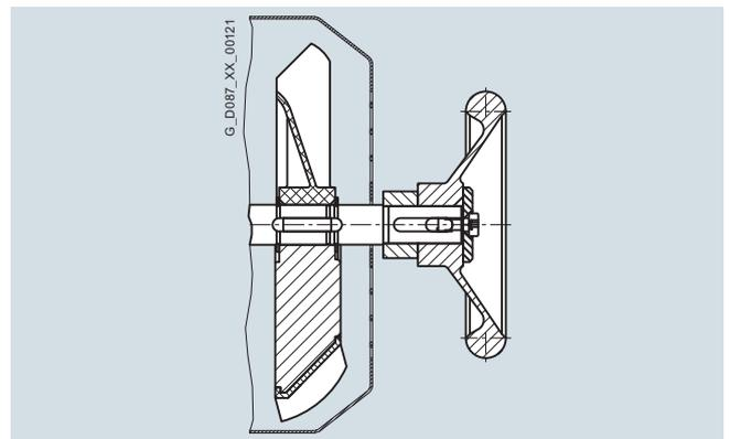
Fig. 11/58 Handwheel
