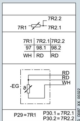
Fig. 10/23 Sensor circuit diagram for Pt100 electrical oil temperature monitoring
