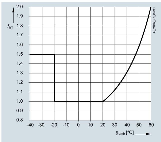
Fig. 2/3 Service factor ambient temperature worm gearbox
