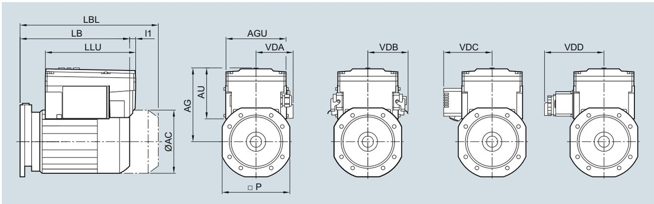
The diagram is for terminal box position 2A (for further information about the terminal box position, see [page 11/16](#)).
