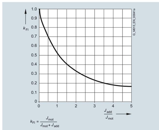
Fig. 2/17 Additional moment of inertia
