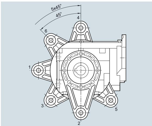
Fig. 10/8 Bevel gearboxes BAD, sizes 19 and 29
