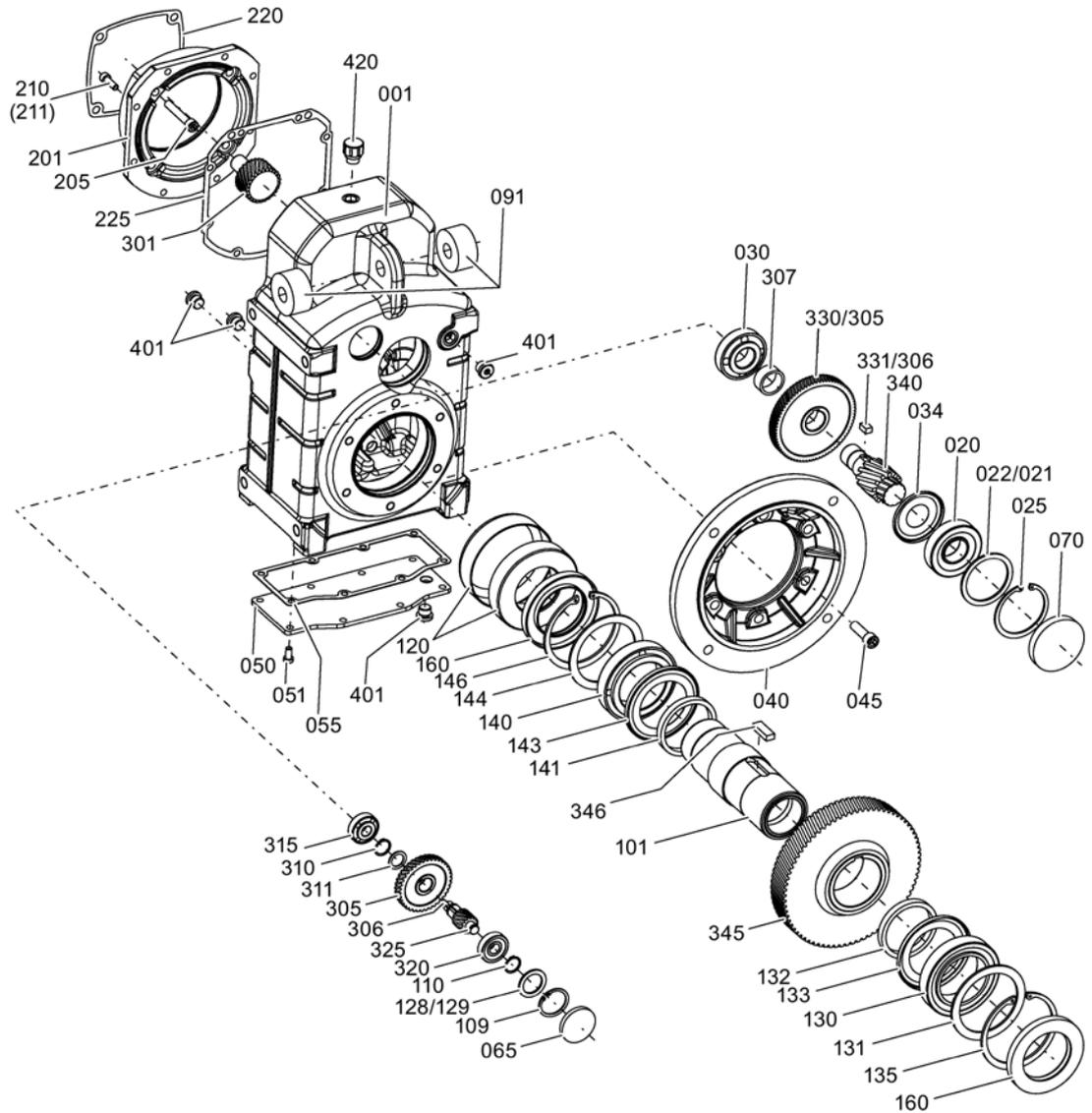
Figure 11-4 Parallel shaft gearbox sizes 38B - 188B
