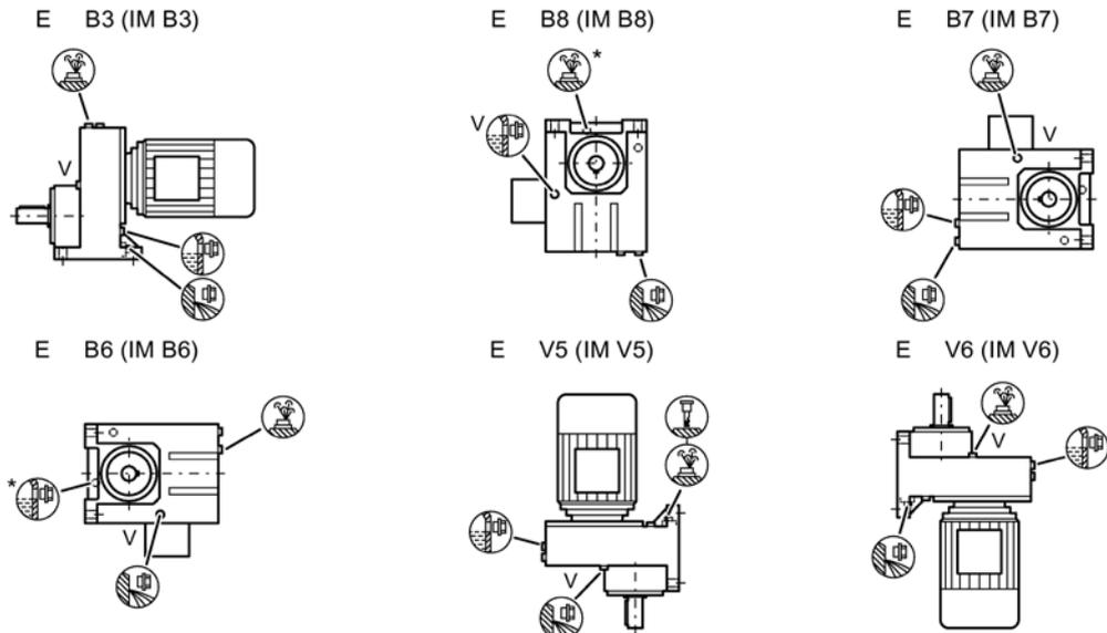
Figure 10-4 Type of construction options for E sizes 38 - 148
