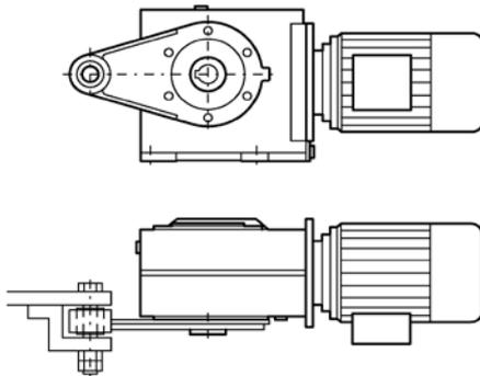
Figure 4-14 Mounting suggestion for torque arm on flange
