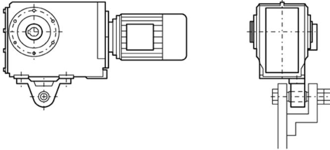
Figure 4-13 Mounting suggestion for torque arm on foot
