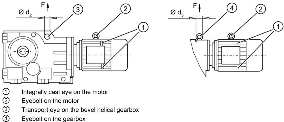
Figure 3-1 Fastening the gearbox or geared motor for suspended transport
