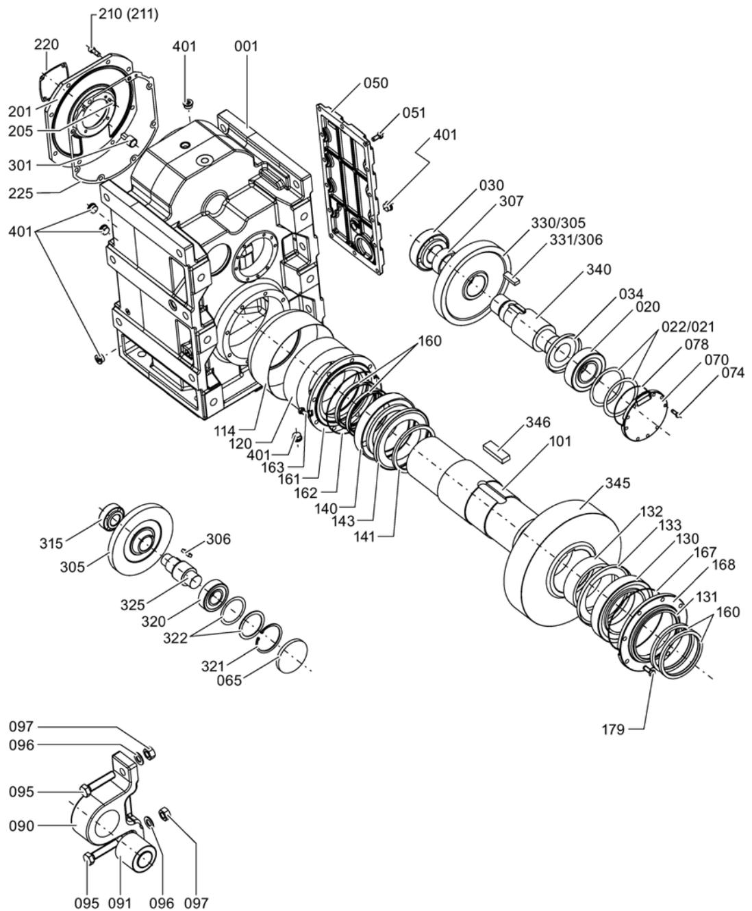
Figure 11-5 Parallel shaft gearbox size 208
