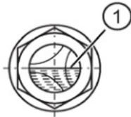
Figure 8-4 Oil level in the oil sight glass
