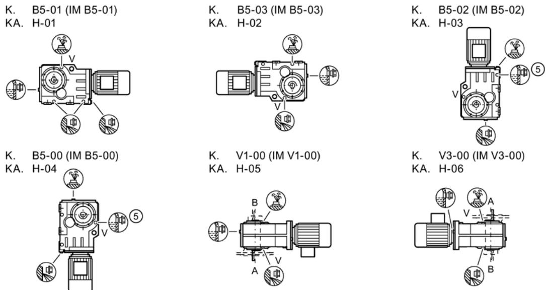
Figure 10-18 Type of construction options for KZ, KF, KM, KAD, KAZ, KAF, KAM, KADS, KAZS, KAFS, KADT, KAZT, KAFT sizes 38 - 188
