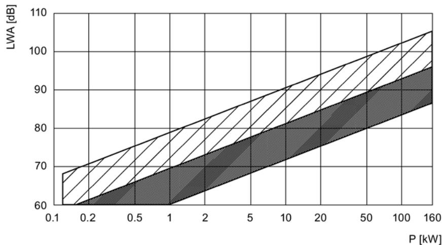
Figure 10-3 Sound energy level MOTOX geared motors
