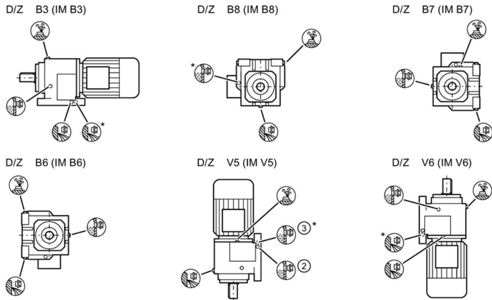
Figure 10-7 Type of construction options for D/Z sizes 108 - 168
