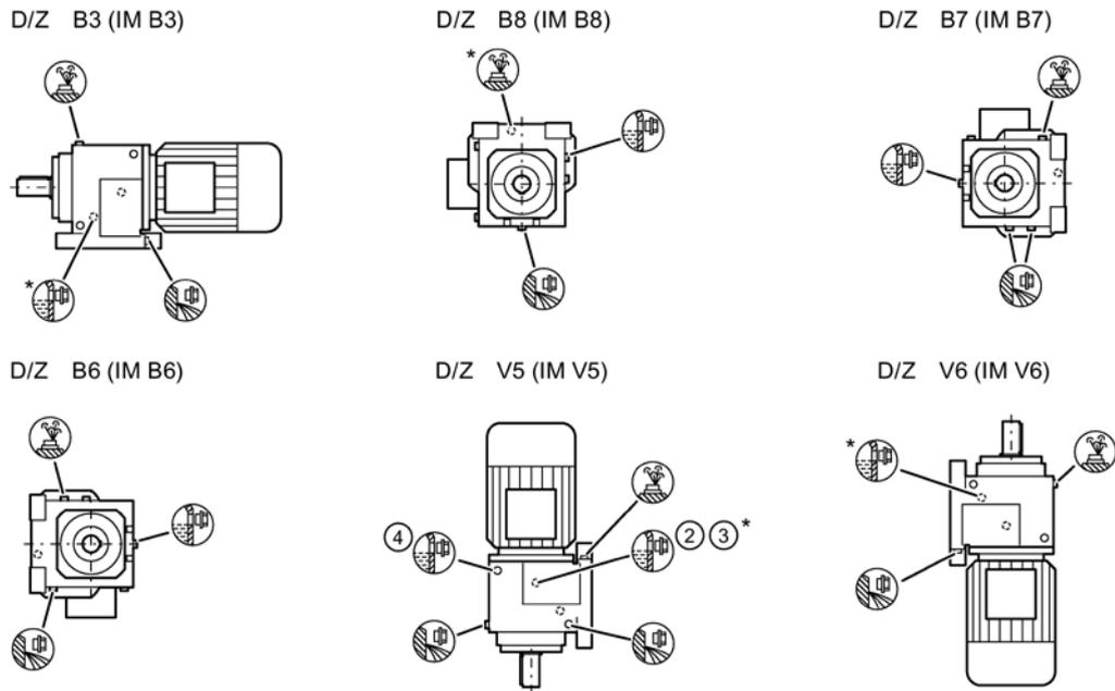
Figure 10-8 Type of construction options for D/Z188
