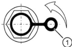
Figure 5-1 Pressure breather valve with securing clip
