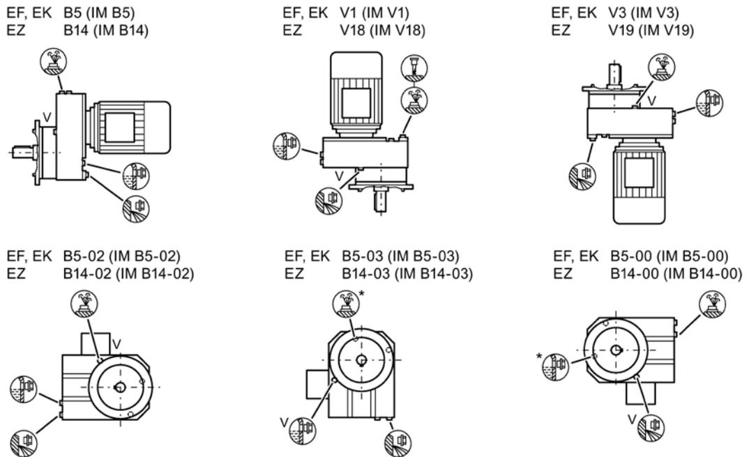
Figure 10-5 Type of construction options for E. sizes 38 - 148
