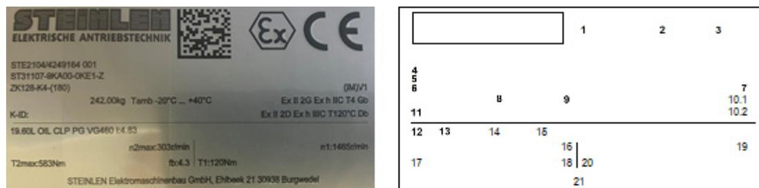
Figure 10-2 ATEX rating plate fitted
