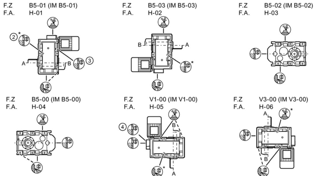
Figure 10-13 Type of construction options for F.208
