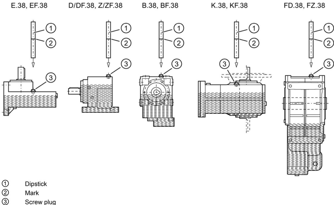
Figure 8-2 Checking the oil level on size 38 gearbox
