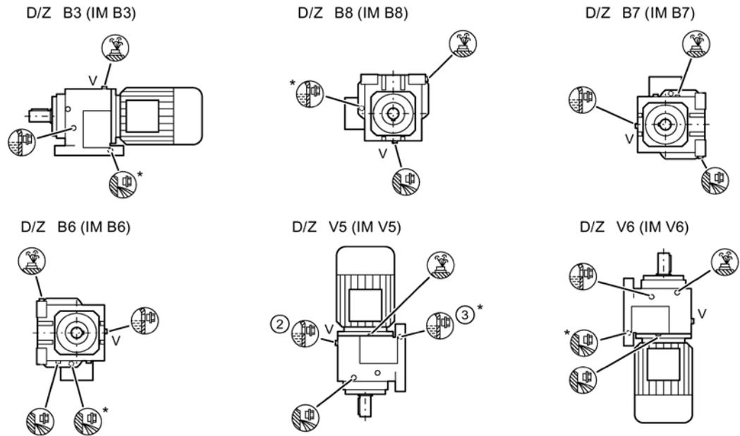
Figure 10-6 Type of construction options for D/Z sizes 18 - 88
