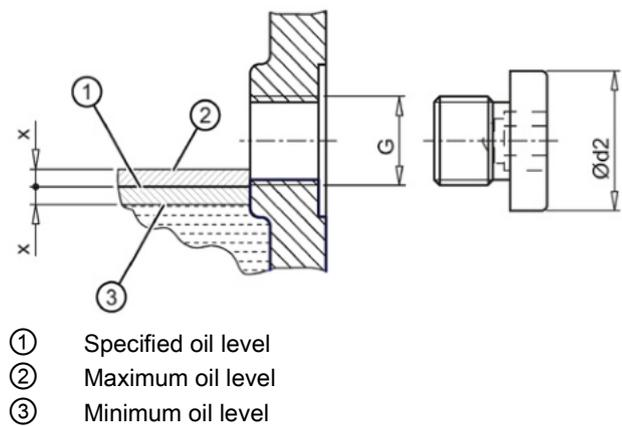
Figure 8-1 Oil level in the gearbox housing
